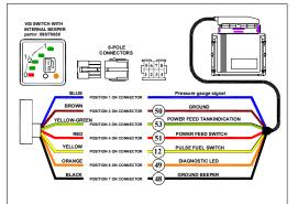
The LPG VSI switch with internal beepers is programmable for different types of tank indicators. Standard setting of the switch is 0-95 Ohm.
