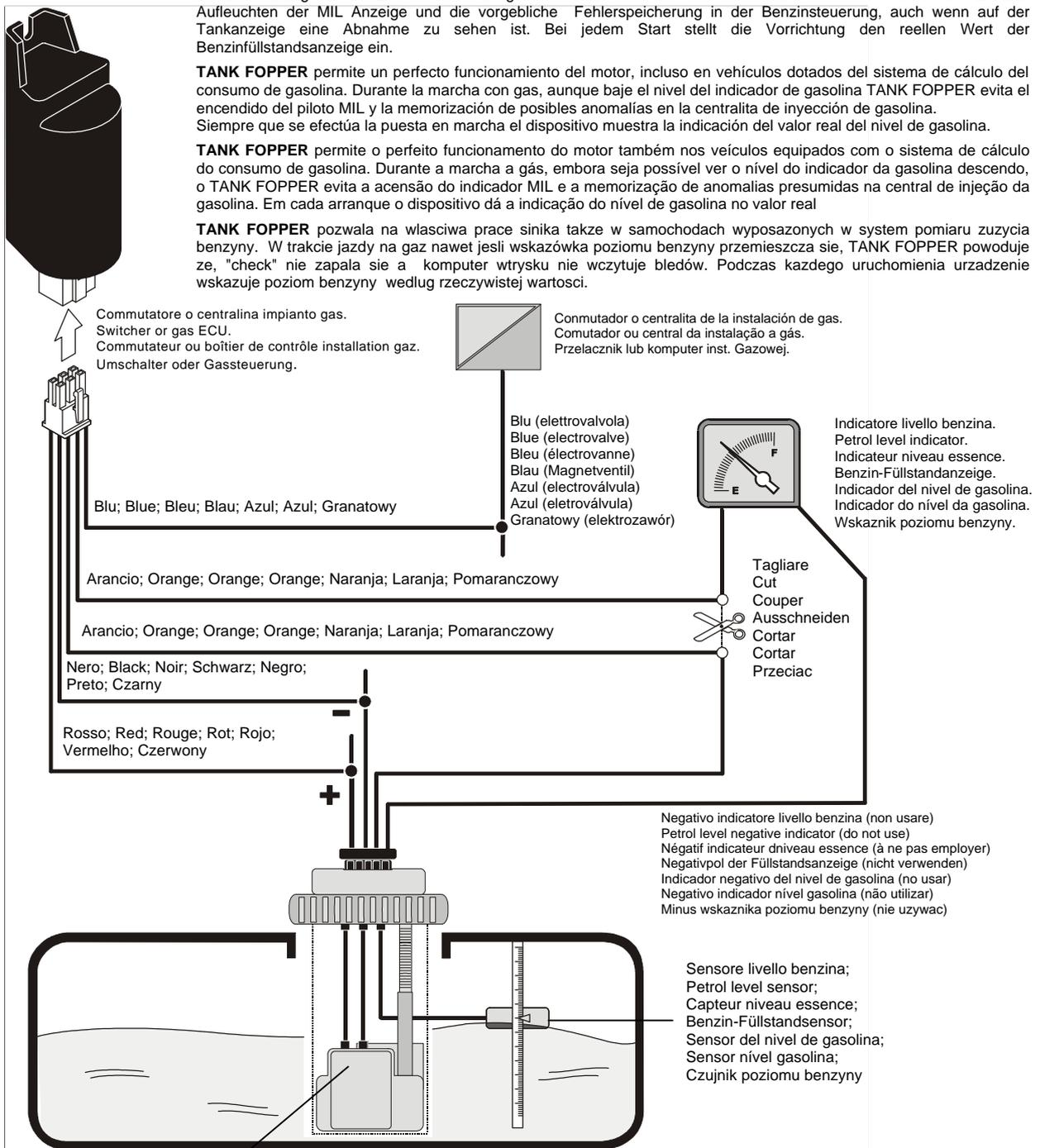
Elettropompa benzina; Electric fuel pump; Electropompe essence;
