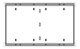
The long frame uses four outer holes (1600mm) and four holes in the center (400mm) for bolt installation
