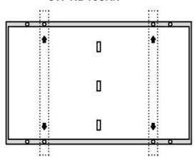
The long frame uses the inner four holes (990mm) for bolt installation
