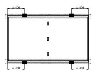
Mounted with 4 clamps along long frame. Mounting bracket/C-shaped steel parallel to the long frame.
