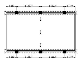
Mounted with 6 clamps along long frame. Mounting bracket/C-shaped steel parallel to the long frame.
