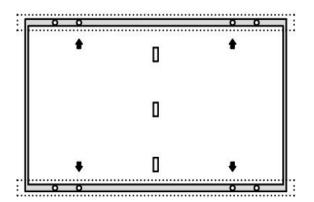
The long frame uses the inner four holes (990mm) for bolt installation
