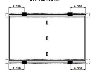
Mounted with 4 clamps along long frame. Mounting bracket/C-shaped steel parallel to the long frame.
