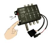
**Step 1:** Start the vehicle and activate gas operation. The dosing module is now provided with power and remains in Set-up ready mode (LED lights up yellow) for 30 seconds.
