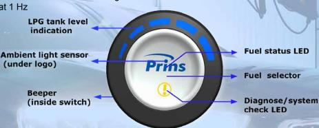
By using the selector switch it is possible to switch between LPG and petrol mode.
