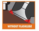
Left valve seats recede into cylinder head resulting in a loss of compression.
