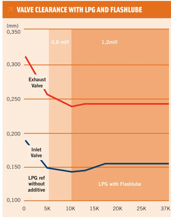
Photos show results of testing with & without Flashlube Valve Saver Fluid
