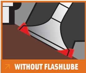
**Left** valve seats recede into cylinder head resulting in a loss of compression.
